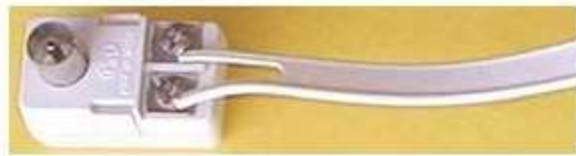
Left is a 300 to 75 ohm balun Right 75 ohm twin lead
